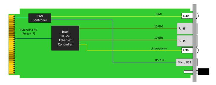
Figure 1: Block Diagram
